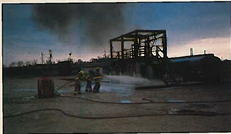
The combination of foam concentrates and flammable liquid runoff have environmental repercussions that merit serious consideration from firefighting management. Above, firefighters at the former Refinery Terminal Fire Company training facility conduct a test burn to create a simulated wastewater condition for treatability testing. At top right, wastewater used in treatability research is contained within a pit, from which samples were drawn by environmental engineers, far right. (Photos by author.)
